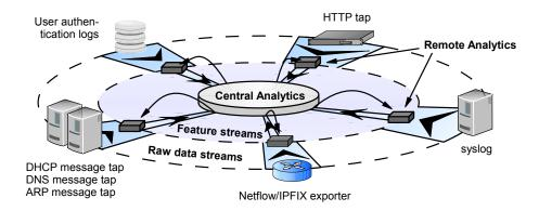
Figure 1: Stream computing for cybersecurity analytics.
