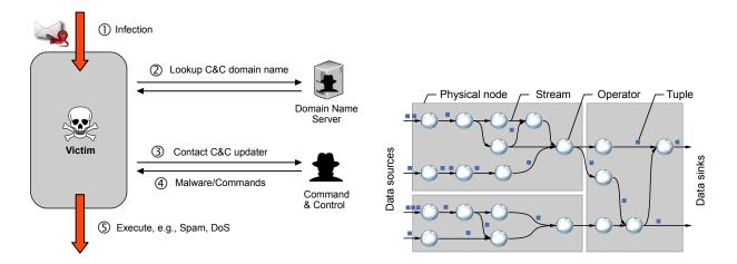
Figure 2: Example of a botnet infection and its command and control (C&C) communication channel.
