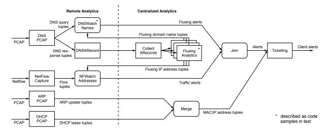
Figure 5: Stream-processing operators in DNS analytics and alerting.
