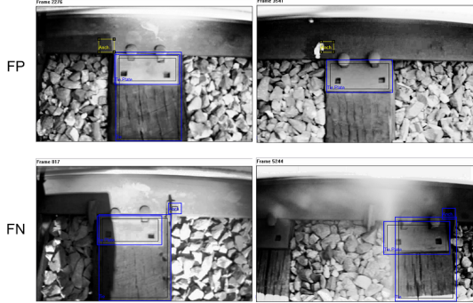
Fig. 15. Examples of anchor false positives (top row) and anchor false negatives (bottom row).
