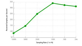
Fig. 2. The number of samples per second received at the collector as the sampling rate increases.
