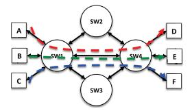
(a) The physical OpenSample testbed with four 10 Gbps IBM G8264 switches configured with 6 hosts and 3 large flows.
