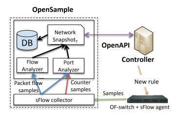
Fig. 3. The architecture of OpenSample providing measurement data to an SDN controller is depicted. sFlow agents running on switches provide samples to an sFlow collector which are then forwarded to flow and port analyzers. This information is aggregated into network snapshots and exposed via an open API. The SDN controller uses this API to make flow rerouting decisions.
