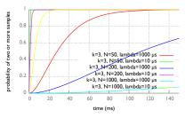
(c) The cumulative distribution function of the delay to get two packets from a flow based on packet inter-arrival rate lambda.
