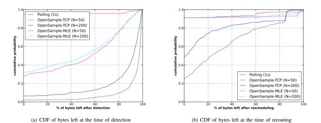
Fig. 6. The percent of bytes remaining in flows at the time of detection and time of rerouting in the Stride8 workload with 1 MB average flow size.
