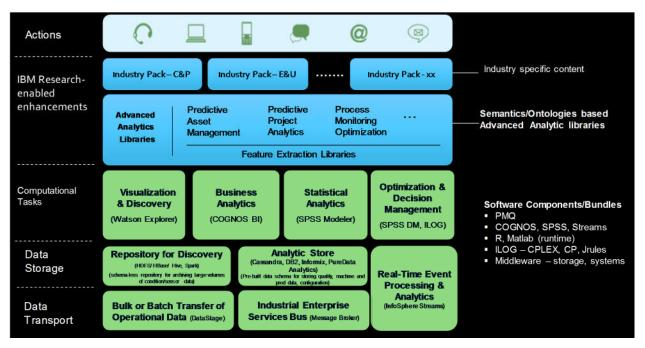
Figure 6: An Architecture for the Semantically defined SROM Analytics Solution
