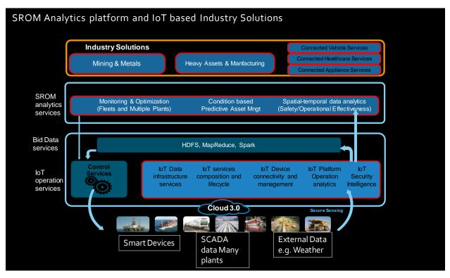
Figure 7: SROM Analytics platform and IoT/Big Data based Industry Solutions
