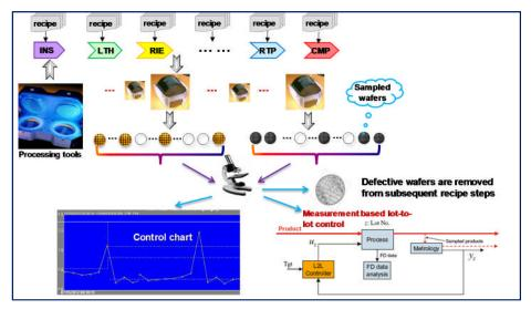
Figure 12: An Illustration of a Predictive Statistical Quality/Process Control Analytics
