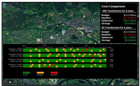
Figure 8: A Sample Output of a Maintenance Planning Optimization Analytics
