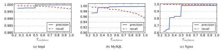
Fig. 6. Configuration file discovery results using vocabulary-based discovery w.r.t. confidence threshold. With a confidence threshold above 0.5, ConfEx's discovery approach achieves above 0.95 precision and recall in all applications we study. Note that the subfigures have different vertical axis scales.
