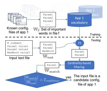
Fig. 4. Discovery phase. A vocabulary is generated for each known application offline. Input text files are compared with each application vocabulary and selected as candidate configuration files upon a match that is larger than a confidence threshold.
