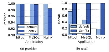
Fig. 7. Comparison of the default path-based and ConfEx's vocabularybased discovery approaches ( $T_{confidence} = 0.5$ ). The default approach can identify only 19-75% of the application configuration files, leading to low recall. ConfEx successfully identifies more than 98% of these files while resulting in less than 2% false positives in Nginx.
