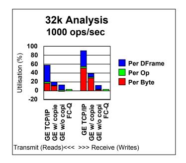
As can be seen, the SCSI over TCP/IP overheads are 30 times higher on reads to the storage device, and 45 times higher on writes to the storage device. When TCP/IP is eliminated, the ratios are 10x and 20x respectively. When copying is also eliminated, the ratios are 7x and 6x respectively.
