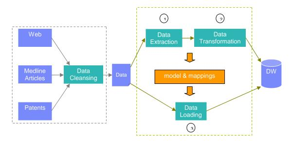
Figure 2. GETL engine architecture.
