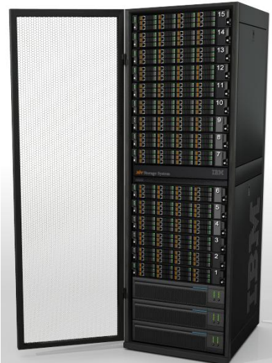
Figure 2: A XIV system with a full rack comprising 15 modules.
