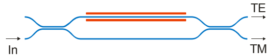
Fig. 6.1: Polarization splitter, based on a symmetric Mach-Zehnder interferometer with trenches etched along one arm.
