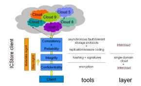
Figure 2: High level design of Intercloud storage.
