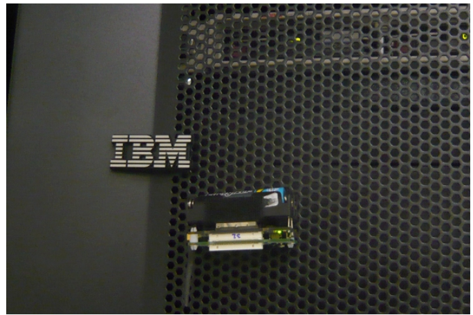
Fig. 2. Wireless sensor node mounted on an IBM server rack to measure the inlet temperature. Magnetic mounting allows for fast and easy deployment.
